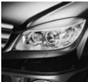
Intelligent Light System Bi-Xenon-Scheinwerfer
